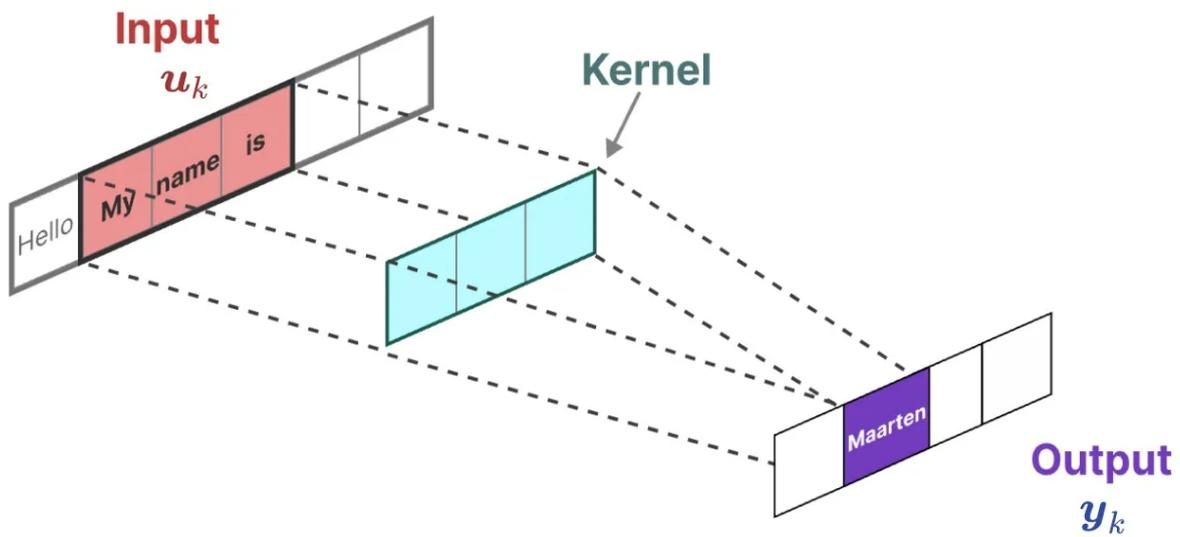
$$\text{kernel} \rightarrow \bar{K} = (\bar{C}\bar{B}, \bar{C}\bar{A}\bar{B}, \dots, \bar{C}\bar{A}^k\bar{B}, \dots)$$
